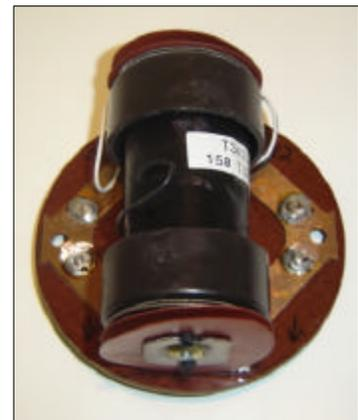
*Finished Coil and Plate Assembly*
